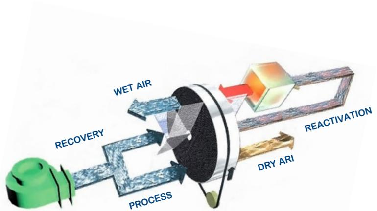
(\*) PTC –Positive Temperature Coefficient- heater or thermistor is a self-regulating semiconductor heating element that dissipates heat according to the air flow in contact with its elements, and this relates directly to the electrical power consumption of the unit. As drying capacity is proportional to reactivation power, by increasing or decreasing the heated air flow we can regulate the drying capacity of the unit. This effect can be clearly observed on the ammeter on the front panel.
